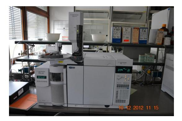
Fig. (3-12): Image of the GC-MS devise at the Geosciences Institute laboratories – Technology University- Darmstadt/ Germany .
