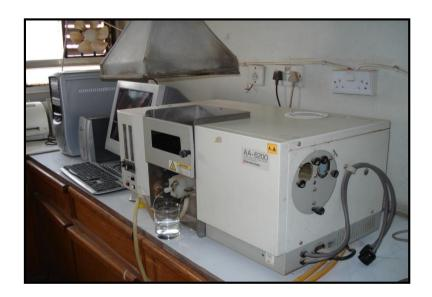
Fig. (3-10): Atomic Absorption Spectrometer (AAS) devise that was used during this study
