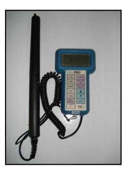
Fig. (3-2): Mono and dioxide carbon (CO, CO<sub>2</sub>) concentrations measuring devise
