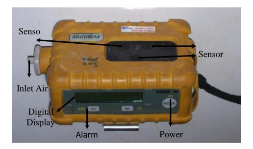
Fig. (3-3): Image of device used in the measurement of (H<sub>2</sub>S, SO<sub>2</sub>, and NO<sub>2</sub>) gases concentrations in the air.
