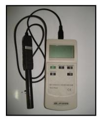
Fig. (3-6): the device that was used for the measurements of air temperature and humidity
